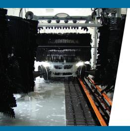
SpinRite's slow-spinning wheels are different. The self-supporting patented ShineMitt media design allows the SpinRite cleaning wheels to spin at 1/3 the speed of traditional car wash equipment, while delivering a superior clean without damage.
